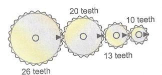
When one gear moves by one tooth, the gear next to it moves by one tooth. The smallest gear moves by one tooth every second.
